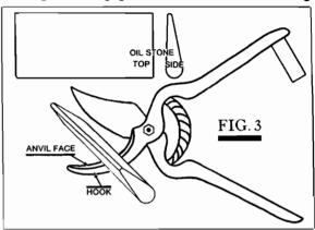
If your pruning shear (Fig. 3), has only one cutting blade, sharpen it as described above. The hook or anvil blade should be cleaned and examined for burs. Remove the burs from the inside face as described above in Figure 1. If the hook face is not nicked, leave it alone. If it is nicked, stone the anvil face (Fig. 3) until the nick is removed. Wipe the shears clean and oil.
