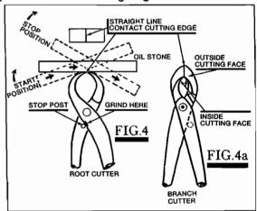
be in a straight line contact (Fig. 4, 4a) or curved line contact (Fig. 5). The condition of contact can be determined by placing the cutter up to the light in a closed position. If a wedge of light shows through, the cutting edges are out of line. If the edges are in line but have very small nicks, proceed to sharpen the tool.
