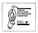
When you first inspect your mandible cutting tools and find an out of line cutting edge condition (Fig. 7) or large nicks, the defects must be corrected prior to sharpening. To line up the cutting edges and remove the nicks, place a six inch strip of 240 grit emery cloth about one and one half times the width of the cutting
